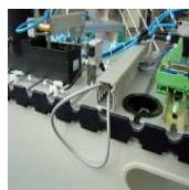
Conductors passing over DIN rails or routed around sharp corners must be secured using 2 cable holders.
