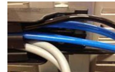
Distance from the shortest pneumatic connection to the first cable tie: 60 mm +/- 5mm Airflow must not be restricted
